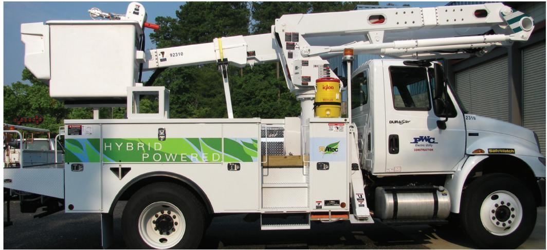
This fall, PWC will introduce their first hybrid bucket trucks into its fleet. Using a Jobsite Energy Management System, the hybrid is designed to fully operate its lift on battery power.
