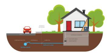
He stated based on knowledge they have in speaking to some of the older retirees, PWC installed galvanized piping from the main to the meter prior to the 1960s. And from the mid-1960s through 2007 PWC installed black plastic polyethylene piping. Since 2007 we installed copper piping from the main to the meter. Installation of piping from the meter to the house has been in accordance with the plumbing code at that time.
