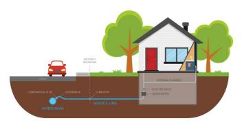
He stated based on knowledge they have in speaking to some of the older retirees, PWC installed galvanized piping from the main to the meter prior to the 1960s. And from the mid-1960s through 2007 PWC installed black plastic polyethylene piping. Since 2007 we installed copper piping from the main to the meter. Installation of piping from the meter to the house has been in accordance with the plumbing code at that time.
