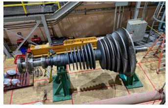
This is a picture of a rotor that was pulled. Experts are brought in to inspect it. It was in good shape, however we needed to clean it. It is cleaned by blasting with ice chips.
