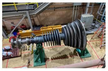
This is a picture of a rotor that was pulled. Experts are brought in to inspect it. It was in good shape, however we needed to clean it. It is cleaned by blasting with ice chips.
