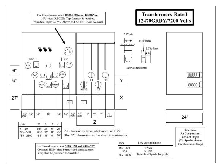
TRANSFORMER, PAD-MOUNT, 3-PHASE, 12KV
